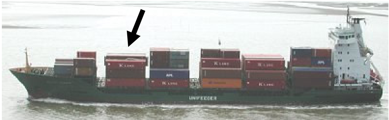
Figure 2.7) Container feeder LoLo-vessel, with a 45ft container stowed on top of a 40ft container. Source: www.containerhandbuch.de (acc: 2004-06-30)
