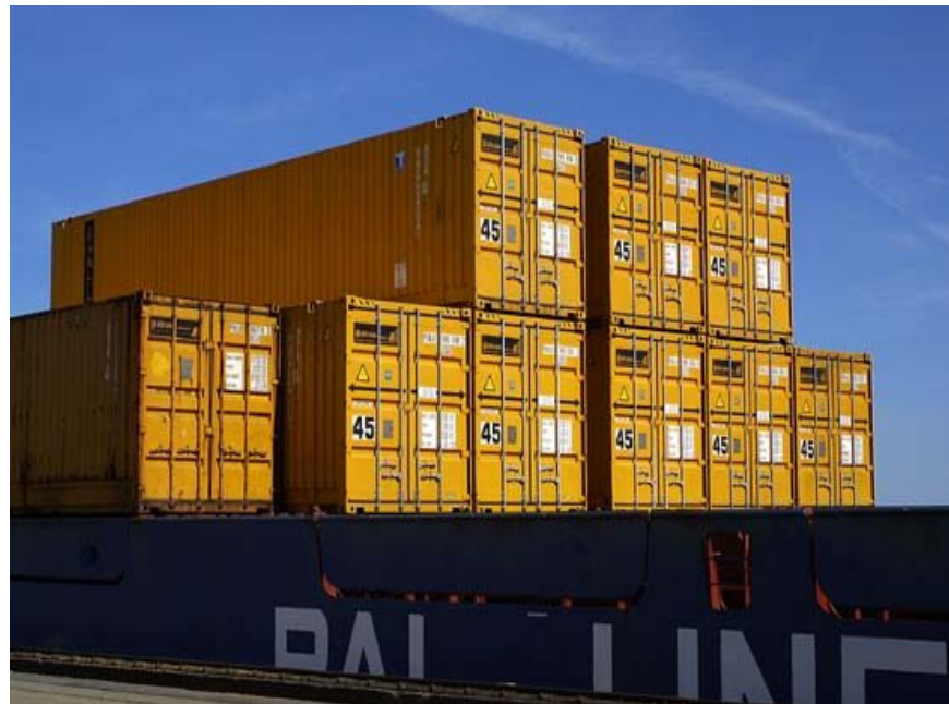
Figure C1-6) 45ft PWHC stowed on deck, source: www.paltrans.se
